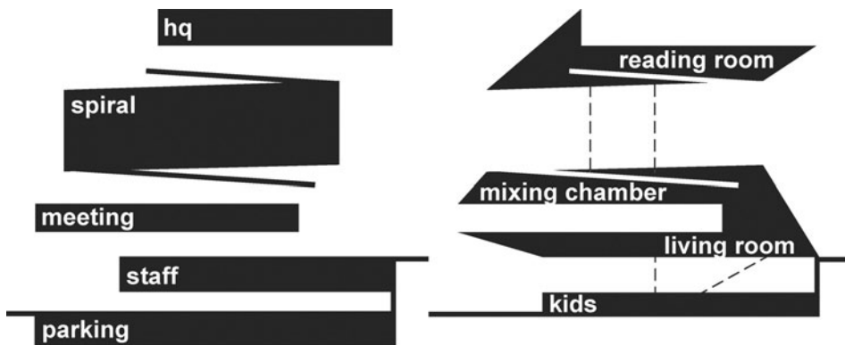
Figure 9.9: Diagrams for floor plate occupancies for the Seattle Public Library showing the platforms (left) and the in-between spaces (right)
